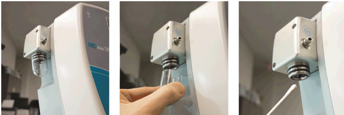
Figure #5 Removing Water Trap Bottle to clean Bottle and Optical Sensor
